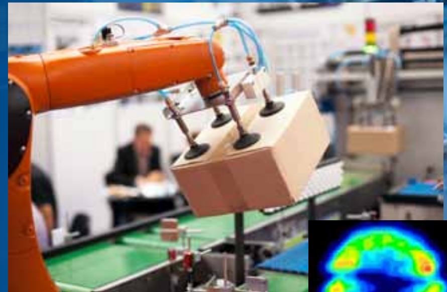
FIGURE 6 PRESSURE MAPPING HELPS TO MEASURE THE PRESSURE DISTRIBUTION ACROSS THE CONTACT AREA OF A COBOT ARM WHILE IT IS IN USE
