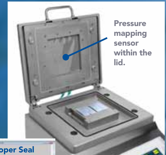
FIGURE 5 THE BONFIGLIOLI PILL PACK MACHINE INCLUDES A PRESSURE MAPPING FEATURE THAT IDENTIFIES LEAKS IN PILL PACKS
